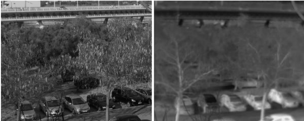
Fig. 2. Two images of the same scene but taken with different cameras one visual camera (left) and one FLIR ThermaCam P20 infrared camera (right)
