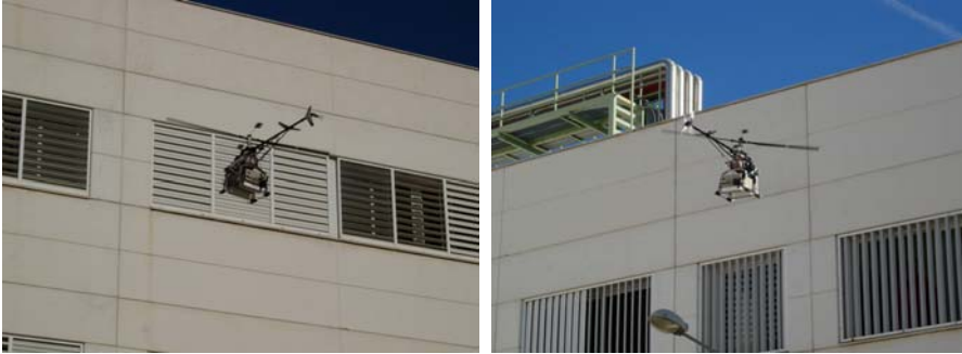
Fig. 10. HERO3 during building inspection experiments carried out at the School of Engineering of Seville (Spain)
