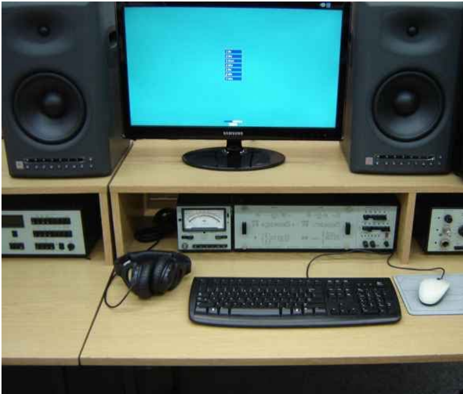
Fig. 9. Speech quality subjective measurement stand.
