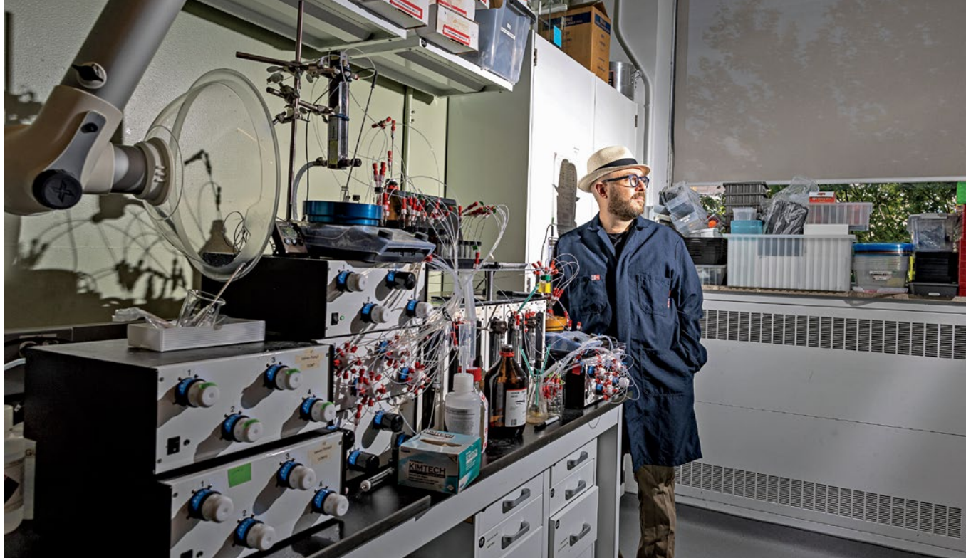
Alán Aspuru-Guzik's lab built Medusa, an open-source, open-design self-driving system for organic synthesis. No experiments were running at the time this photo was taken, and the equipment was turned off.
